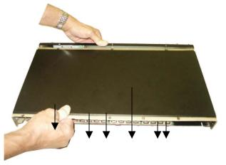
Fig 3.5.1b: Pulling out the top coved from the chassis base
